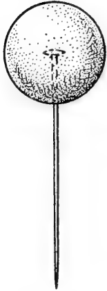
Fig. 11. — NAPHTHA- LENE CONE. Made with a moth ball and com- mon pin.
